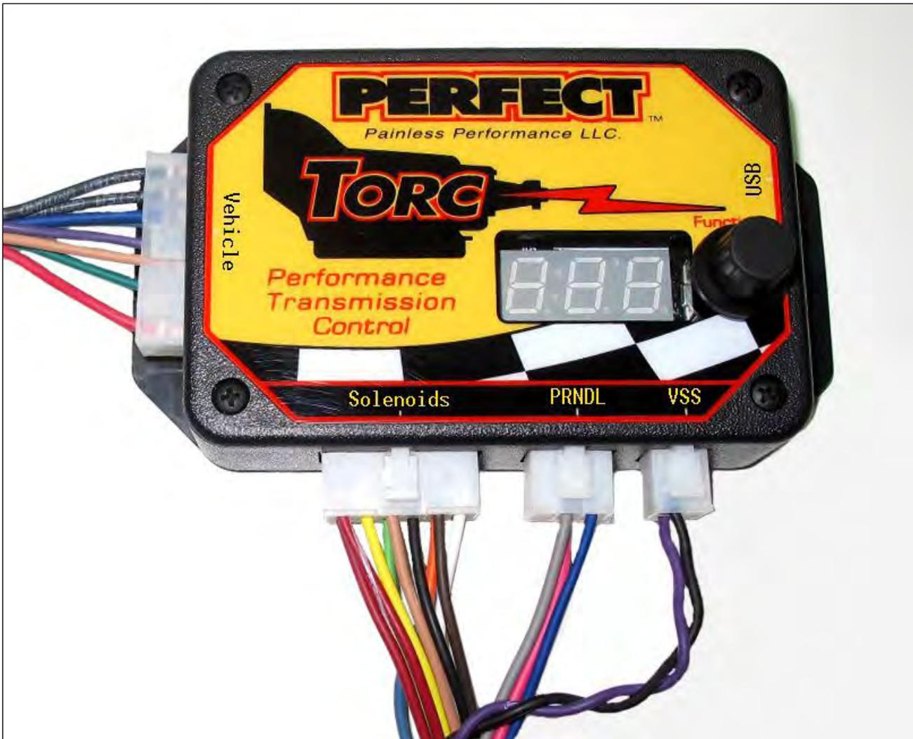
**Figure 2 – Transmission Harness Connections on TORC Module**
