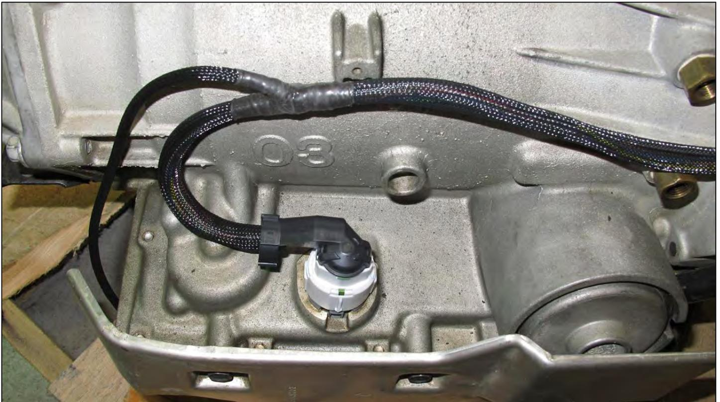
**Install Picture 1 – Main Transmission Connector**
