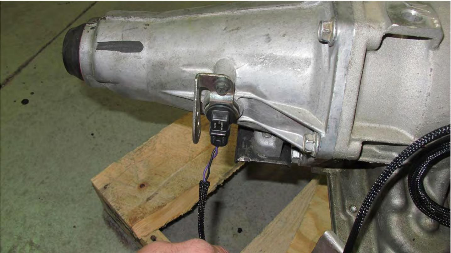
Install Picture 2 – VSS (Vehicle Speed Sensor) Connector
